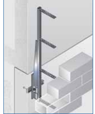
Supports in the Attic with Attic Brickwork Support JAV and JMA (see page 34)
