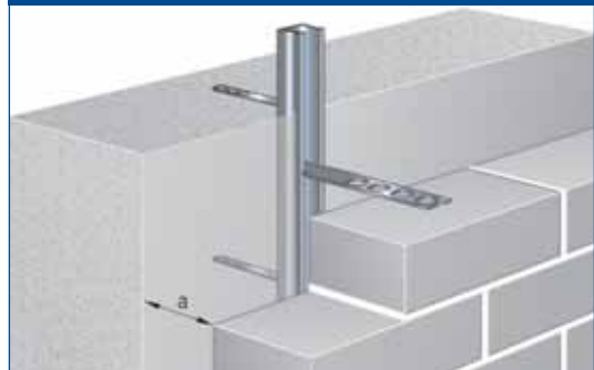
Connection of Facing Shells to Reinforced Concrete Components with Brick Tie Channels Kt 28 / 15-D and Brick Ties
