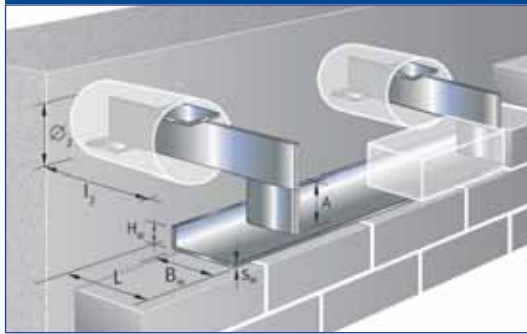
Grout-in Bracket JMK+ FAR
