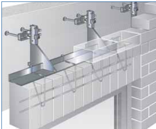
Hidden support over a window openings with JVA+ F and suspension loop
