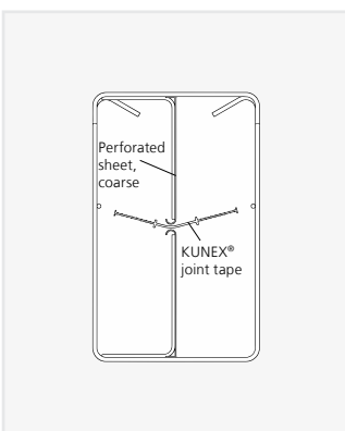
KUNEX® ABS-R floor/floor (ceiling/ceiling) coarse joint.
