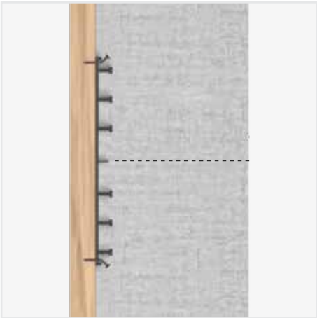
Wall-wall construction joint: Attachment to the formwork.
